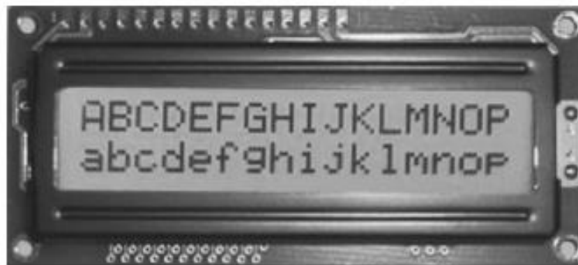
Fig. 8.46 A common 2 × 16 alphanumeric LCD module
